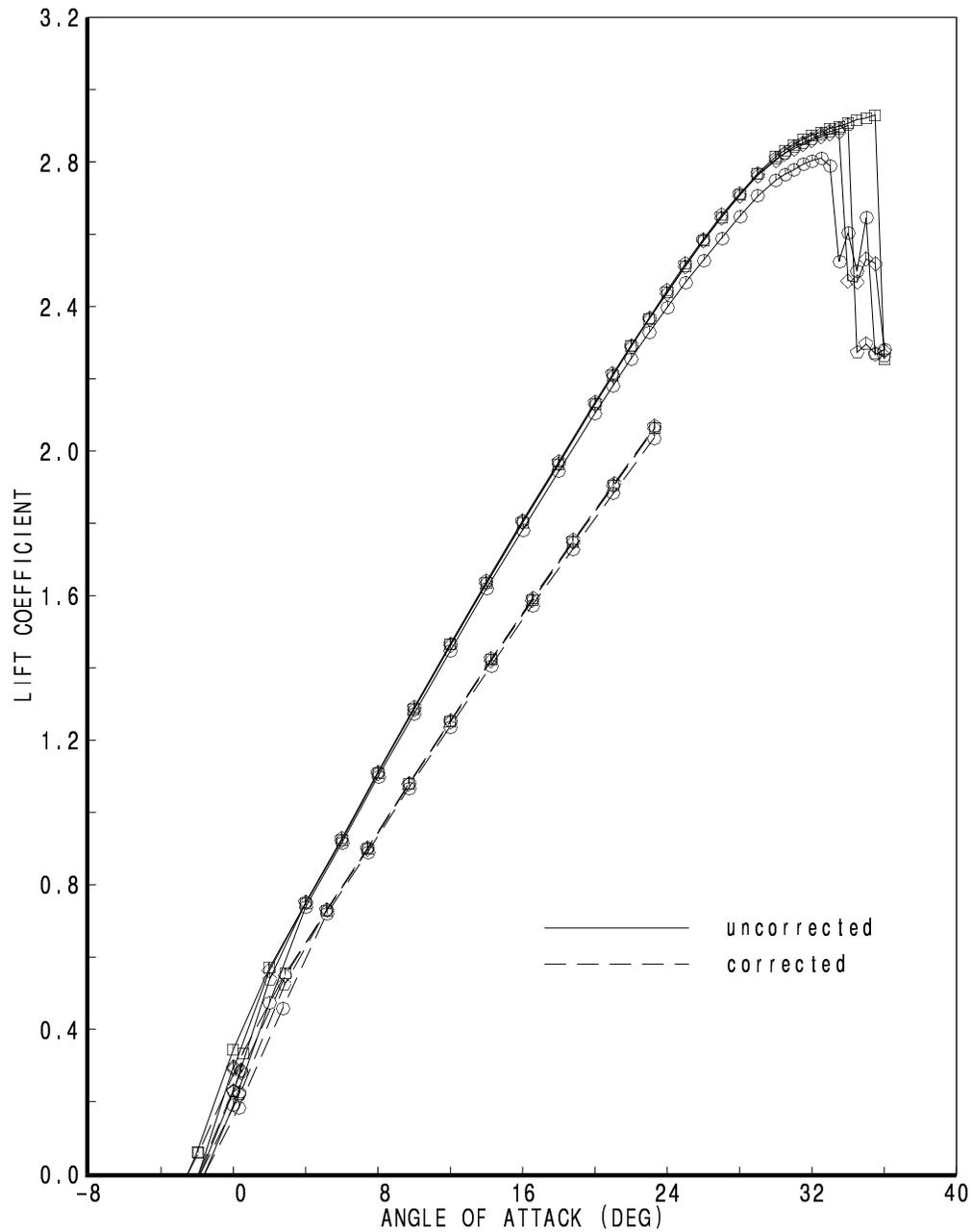
**Part-Span Landing, Configuration 44**
