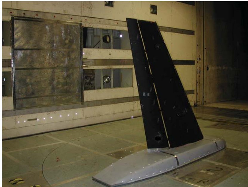
Figure 1. Photograph of the Trapezoidal Wing in the NASA Langley 14x22 Foot Tunnel.
