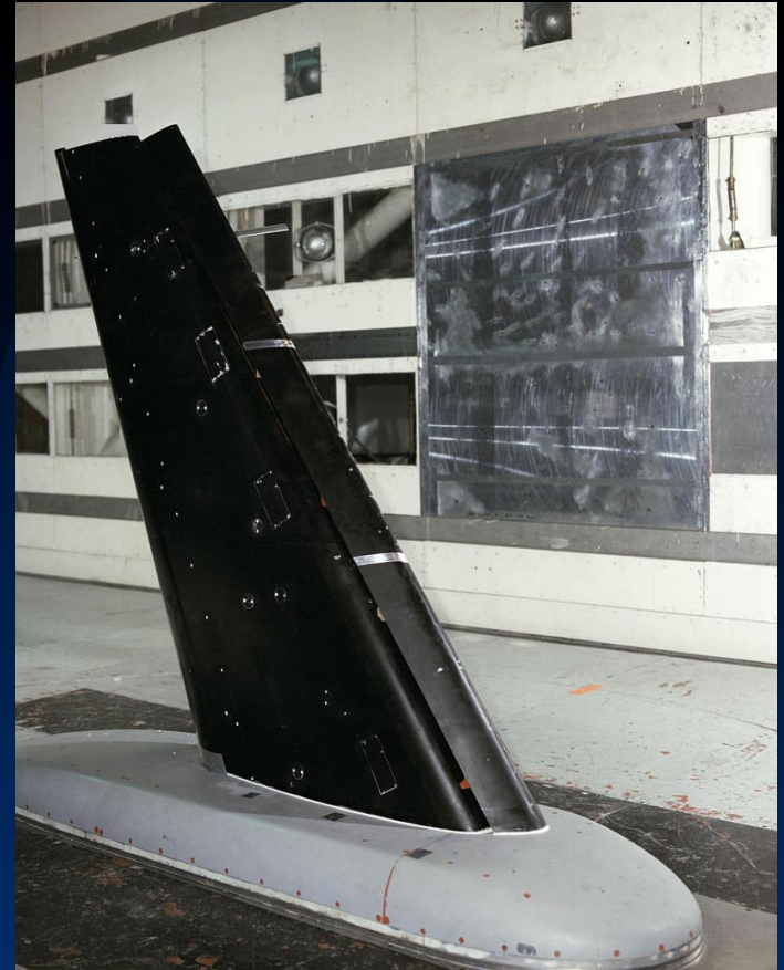
Trap wing in NASA LaRC 14x22 WT
