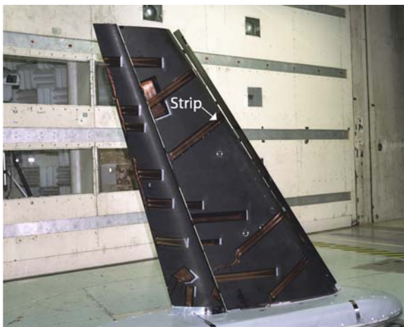
Figure 1. Trap Wing model in 14 x 22 wind tunnel, model upper surface shown.
