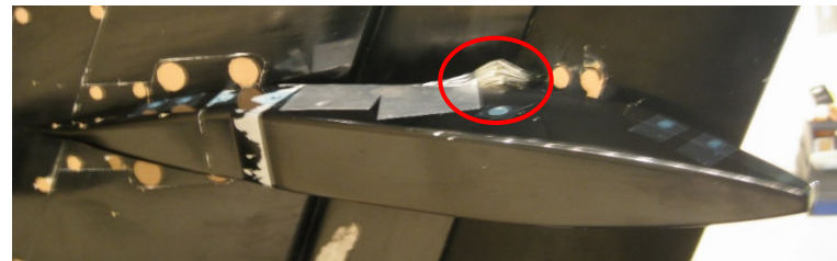
2. The flap support and static pressure tubes are covered by FTF.
