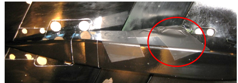
3. Protruded pressure tubes are covered by tape.
